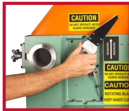
The Quick Blade-Change System is standard on the INTELLICUT® and optional on the SMARTCUT®.
