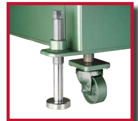
Height Adjusting Casters are standard on the INTELLICUT® and optional on the SMARTCUT®.
