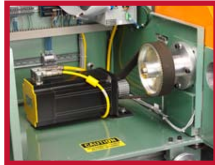
The Servo-Drive produces superior repeatability and more accurate cutting.
